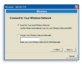
In the Infrastructure mode, you have to allow the Print Server to associate with an access point. You can choose to let the Print Server scan for an available access point automatically, or you can manually assign the SSID of the access point you want to use.
